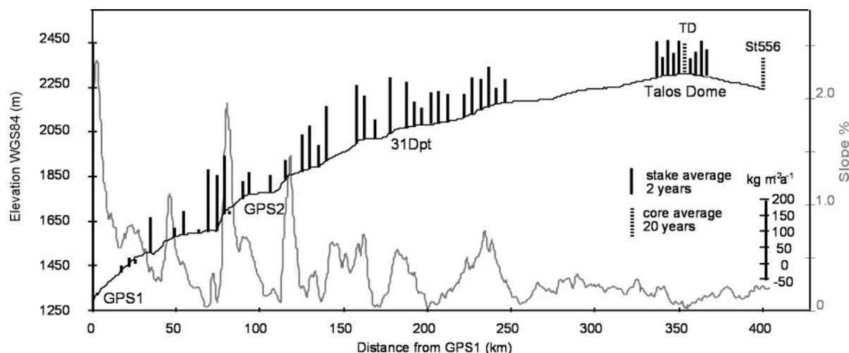
Fig. 6 - Surface mass balance, elevation (solid line) and slope (grey line) along the GPS1-Talos Dome traverse. Surface mass balance is expressed as bars on a cross-sectional profile of the ice sheet. Positive values have been plotted on the ice sheet surface and negative values below the surface. Dash bars at TD and ST556 sites show snow accumulation from firm core analysis (Stenni et al., 2002).
