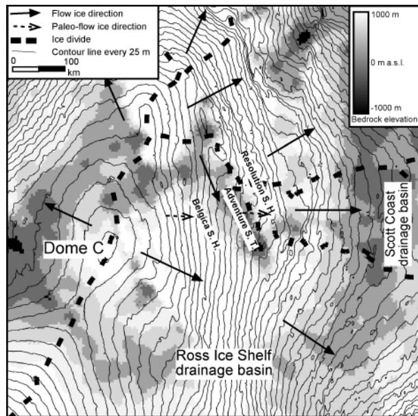
Fig. 3 - Western Scott basin ice divide along the Terra Nova Bay-Dome C traverse. Contour line every 5 m (Rémy et al., 1999), bedrock elevation (gray image, from Lythe et al. 2000 redraw), flow direction, ice divide (Frezzotti et al., 2000) and paleo-flow direction reconstructed using re-constructions of Last Glacial Maximum flowlines (Denton & Hughes, 2000, redrawn).
