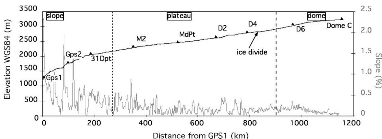
Fig. 2 - Surface elevation (solid line) and terrain slope (grey line) along Terra Nova Bay-Dome C traverse. Core locations are indicated with triangles.
