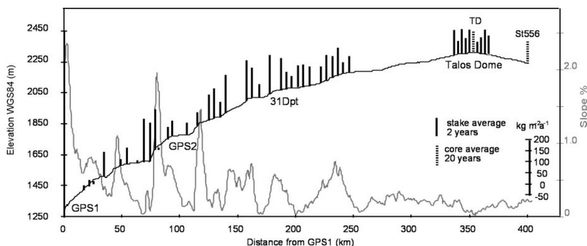
Fig. 6 - Surface mass balance, elevation (solid line) and slope (grey line) along the GPS1-Talos Dome traverse. Surface mass balance is expressed as bars on a cross-sectional profile of the ice sheet. Positive values have been plotted on the ice sheet surface and negative values below the surface. Dash bars at TD and ST556 sites show snow accumulation from firm core analysis (Stenni et al., 2002).
