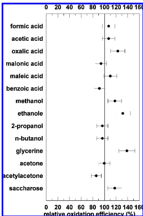
**FIGURE 3.** The oxidation efficiencies of different organic molecules relative to the potassium hydrogen phthalate (PHP) TOC standard (set to 100%). For each molecule three different dilutions in the concentration range of 20–130 ppbWC were measured. Shown error bars of  $\pm 10\%$  are larger than the resolution of the system, because they include the uncertainties introduced by the dilutions of the pure chemical substances.
