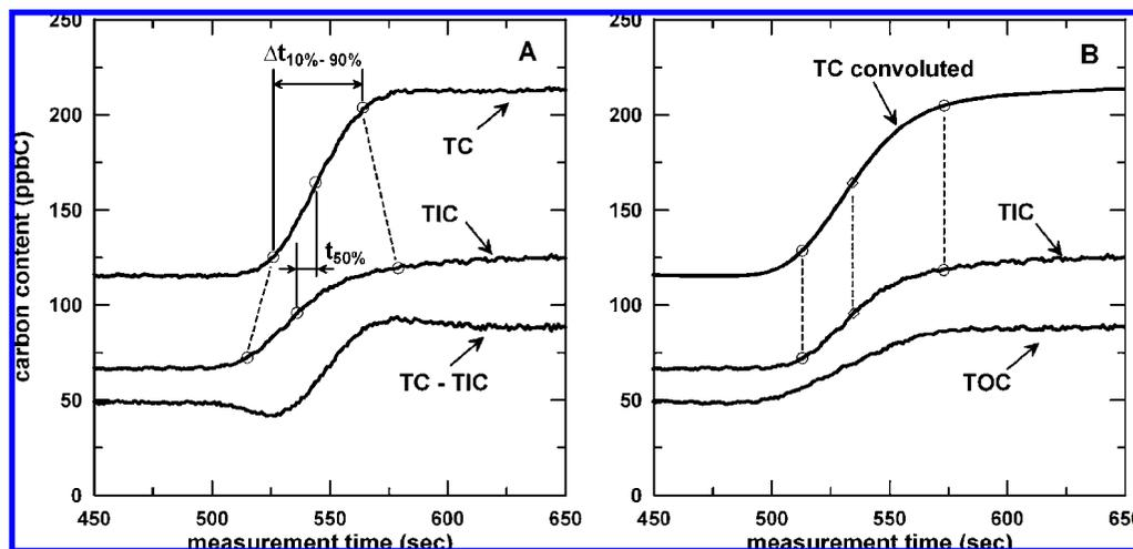
FIGURE 2. Example of the measurement of a 39 ppbC TOC standard. (A) Data of TC and TIC without correction, together with the difference TC-TIC. Under- and overshooting of the difference signal are clear artifacts caused by an insufficient synchronicity of the TC and TIC signals (B) Convoluted TC signal and the resulting TOC data.
